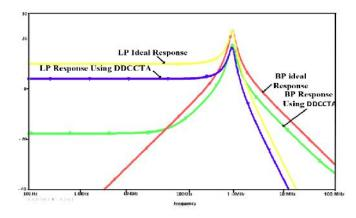
Fig.13 Response of TT configuration of Fig.12 (a) and ideal resonse
