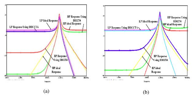
Fig. 9. (a) Magnitude Response of Fig. 8 (a) compare to ideal response (b) Magnitude Response of Fig. 8 (d) compare to ideal response
