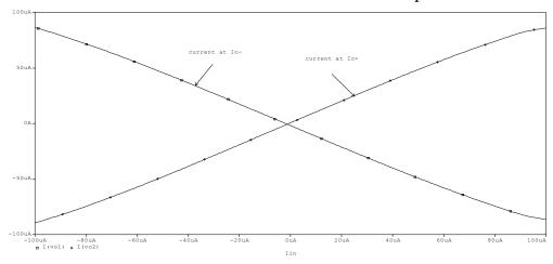
Fig. 6. DC transfer characteristic for current transfer from X port to O+ and O-
