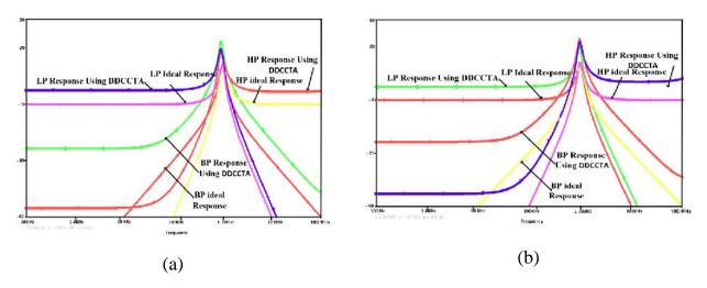
Fig. 10. (a) Magnitude Response of KHN type B class I compared to ideal response (b) Magnitude Response of KHN type B class IV compared to ideal response
