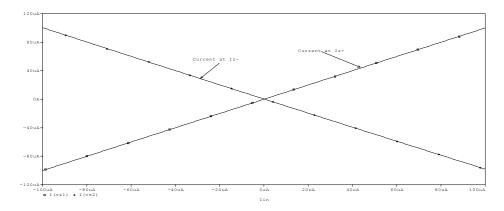
Fig. 5. DC transfer characteristic for current transfer from X port to Z+ and Z- Ports.
