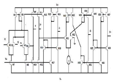
Fig. 2. The CMOS realization of modified DDCCTA [10]
