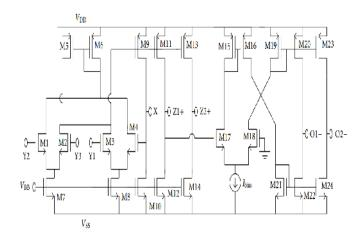
Fig. 1. The CMOS realization of the DDCCTA[10]
