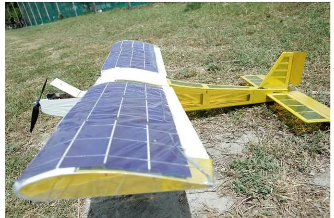
FIG. 5 SOLAR RC AIRCRAFT
