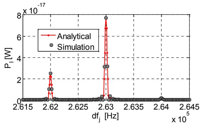
Figure 7-b: Correlator output power for CWI in the case of satellite-2.
