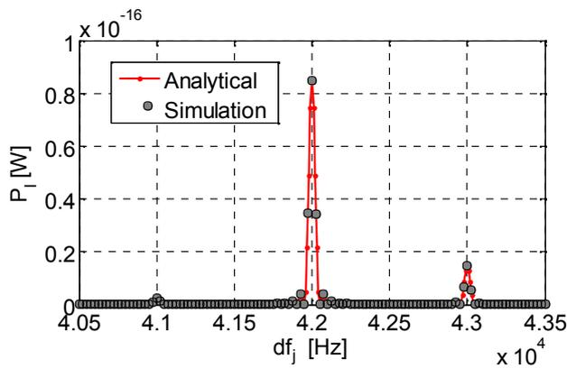
Figure 7-a: Correlator output power for CWI in the case of satellite-1.
