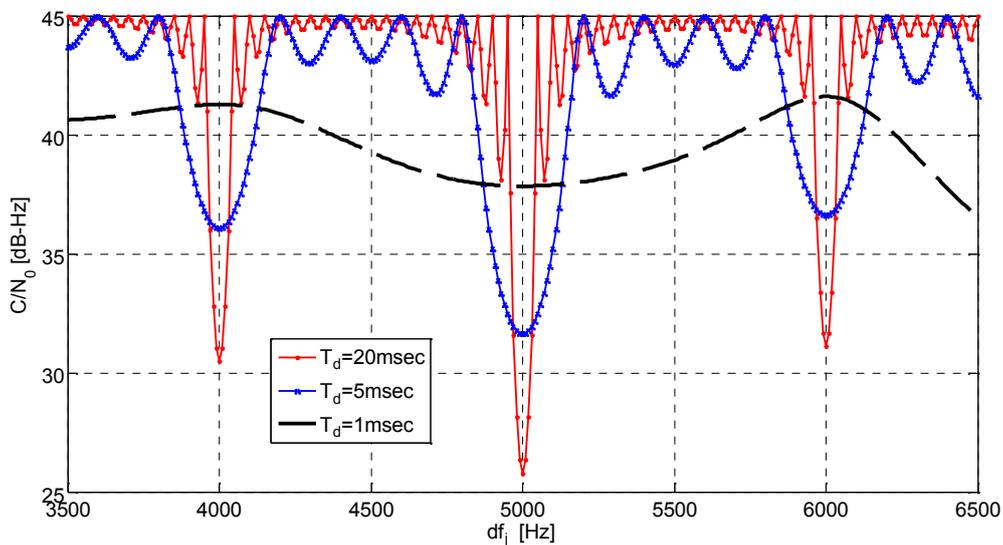
Figure 4: the post-correlation C/No in the presence of CWI at different  $T_d$ .
