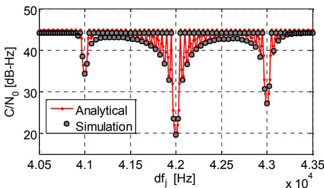
Figure 8-a: C/No in presence of CWI in the case of satellite-1.
