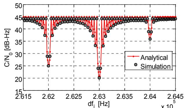
Figure 8-b: C/No in presence of CWI in the case of satellite-2.
