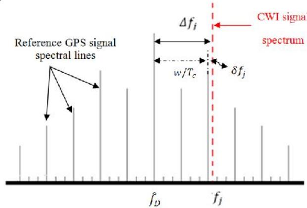
Figure 1: The reference GPS and CWI signals spectrum.
