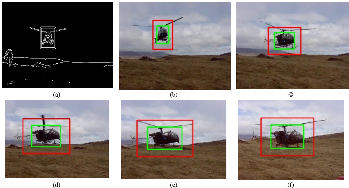
Fig.9 Target tracking result for a sequence; (a) frame No. 25 shows canny edge detection technique on the image, (b) frame No. 100, (c) frame No. 150 (d) frame No. 200, (e) frame No. 250, (f) frame No. 325.
