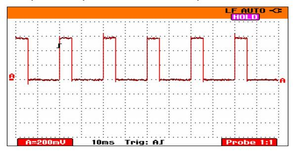
Figure 8: The output pulses waveforms from the optical rotor transducer
