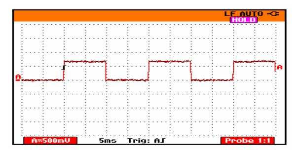
Figure 10: The output pulses from the zero detecting circuit of the bus bar voltage
