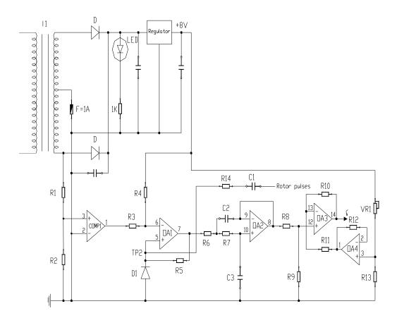
Figure 3: Circuit diagram of the power angle device
