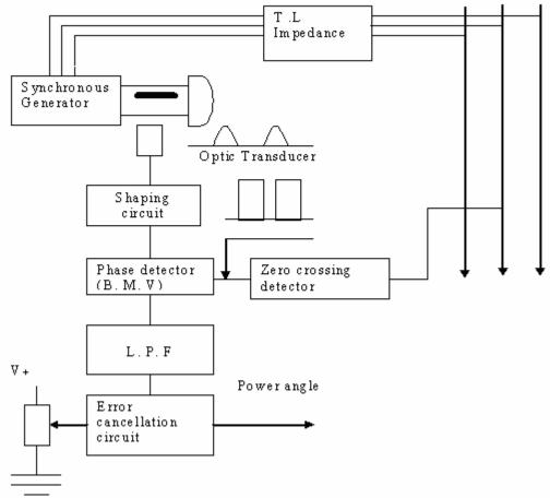
Figure 2: Block diagram for forming the power angle
