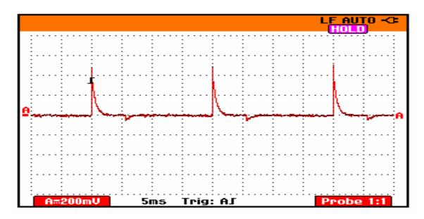
Figure 9: The differentiated rotor transducer pulses
