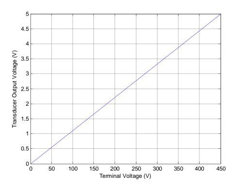
Figure 17: The terminal voltage transducer output voltage curve.
