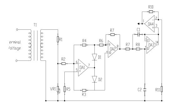
Figure 7: Circuit diagram of the terminal voltage transducer
