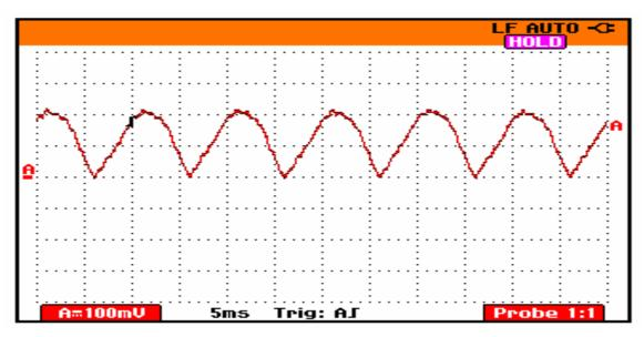
Figure 14: The output from the full-wave precision rectifier circuit
