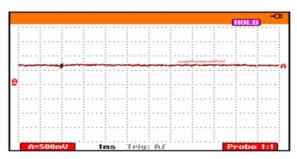
Figure 12: The DC output voltage equivalent to the power angle
