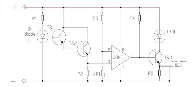
Figure 1: Circuit diagram of the optical transducer
