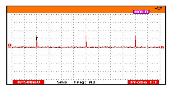
Figure 11: The power angle pulses at no load
