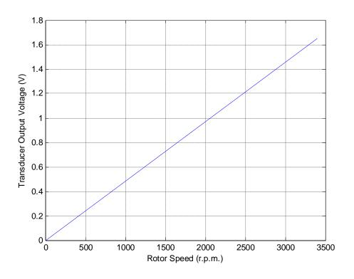
Figure 6: The rotor speed transducer output voltage curve
