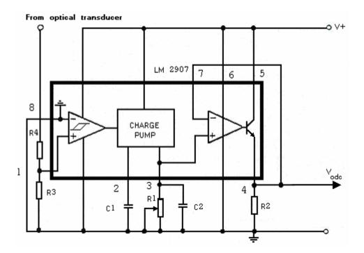
Figure 5: Circuit diagram of the rotor speed measuring unit.
