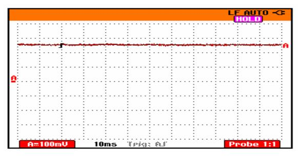
Figure 15: The output of the low pass filter of the terminal voltage transducer
