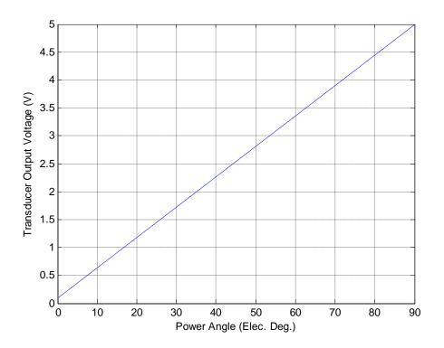
Figure 16: The power-angle transducer output voltage curve
