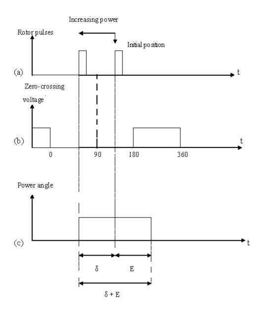
Figure 4: Pulse waveform for generating the power angle
