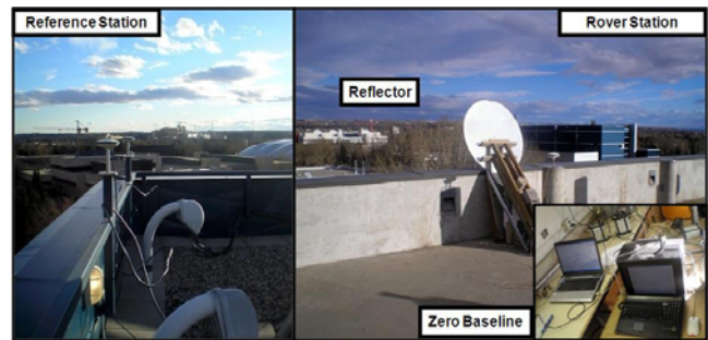
Figure 1. Reference and rover antennas, tow receiver at the rover setup.
