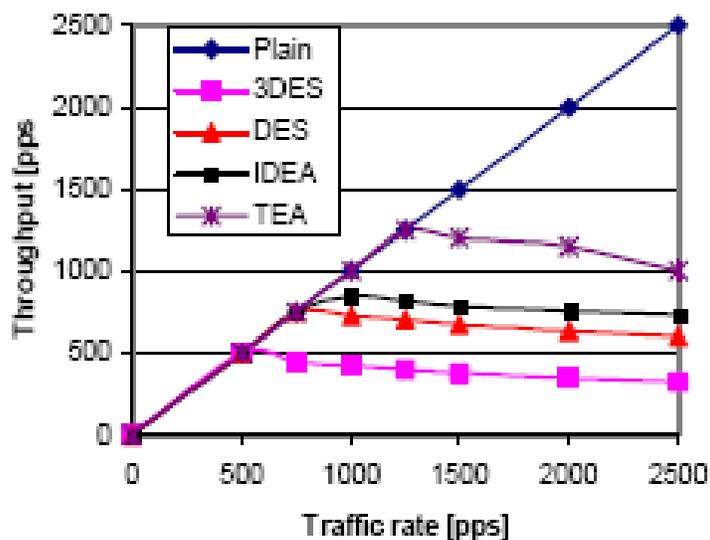
Figure (3): Throughput of the crypto-engine in pps as a function of linearly increasing traffic in pps for plain and encrypted traffic
