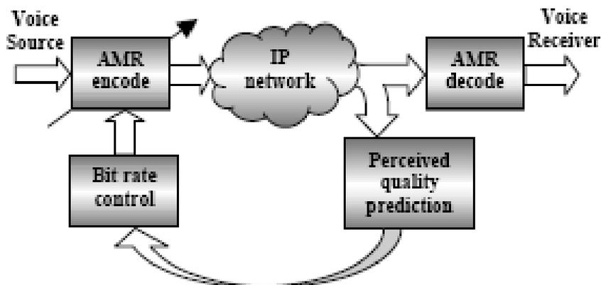
*Figure (1): Rate-adaptive QoS control scheme*
