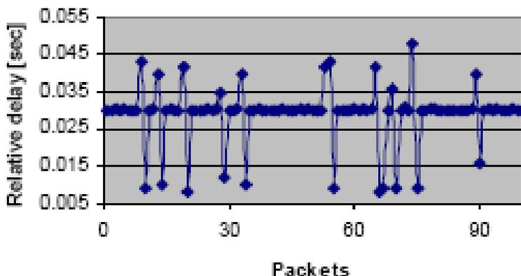
**Figure (4-c):** Individual packet interarrival time for voice traffic when adapting to both network conditions and end-point CPU capability
