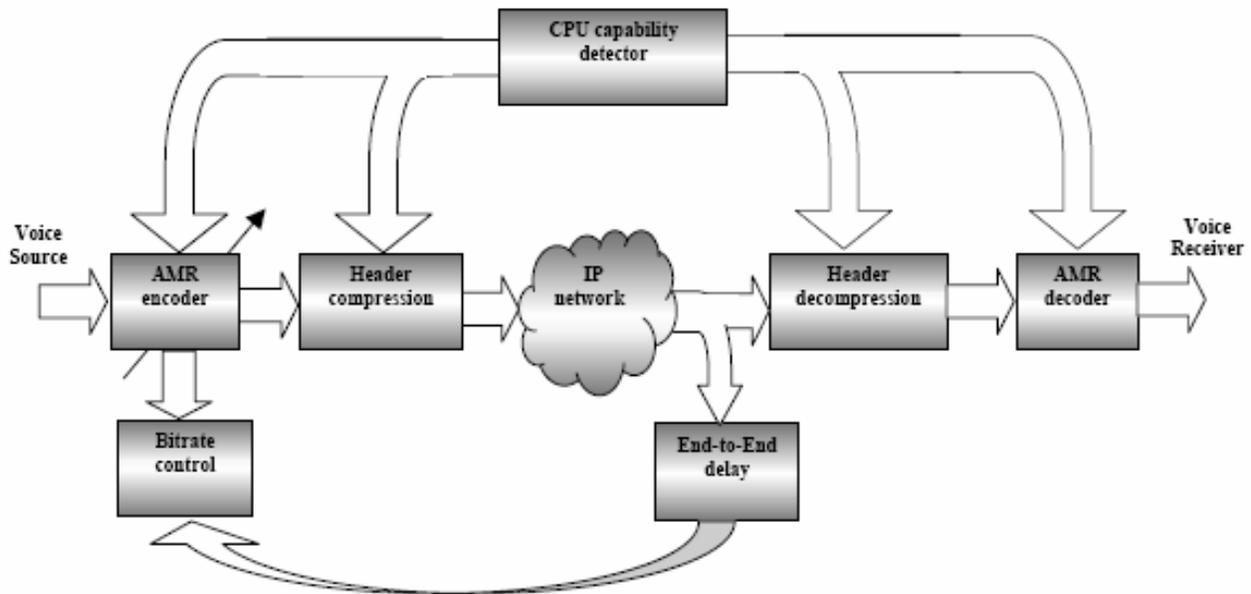
*Figure (2): Proposed adaptive QoS Control Scheme*
