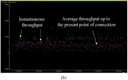
Figure (4): (a) LA process (b) Corresponding TCP throughput
