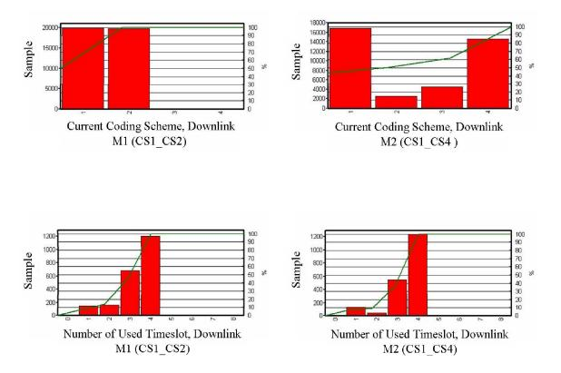
Figure (6): Overall downlink current coding scheme usage and time slot allocations
