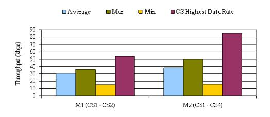
Figure (2): Client downlink overall throughput
