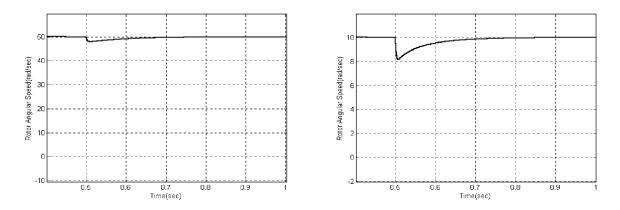
Fig. 9 Responses for sudden loading the motor from no-load to full-load torque, initial steady state speeds of ,(a) 50 rad/s, (b) 10 rad/s
