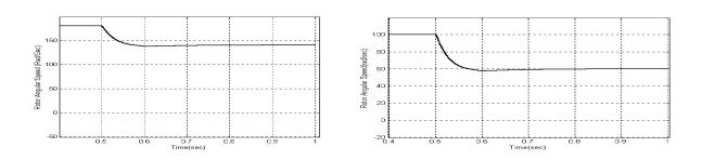
Fig6 Responses for a step decrease in speed reference amount to 40 rad/s , for initial steady state speeds of, (a) 180 rad/s ,(b) 100rad/s
