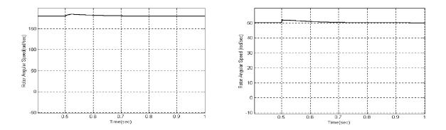
Fig.8 Responses for sudden unloading the motor from full-load to no-load torque, initial steady state speeds of ,(a) 180 rad/s, (b) 50 rad/s
