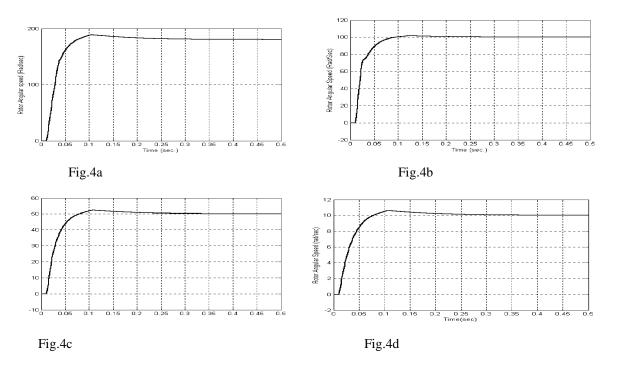
Fig. 4 Responses for step increase in speed reference from standstill and at no-load torque, (a) for 180 rad/s,(b) for 100 rad/s, (c) for 50 rad/s, (d) for 10 rad/sand.
