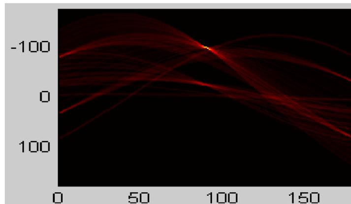
Fig.4 Hough transform of a sample scratch defect
