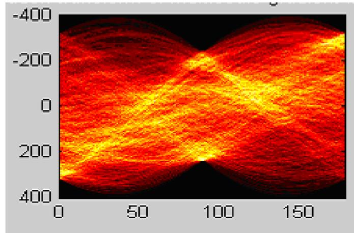
Fig.3 Hough transform of a sample hole defect
