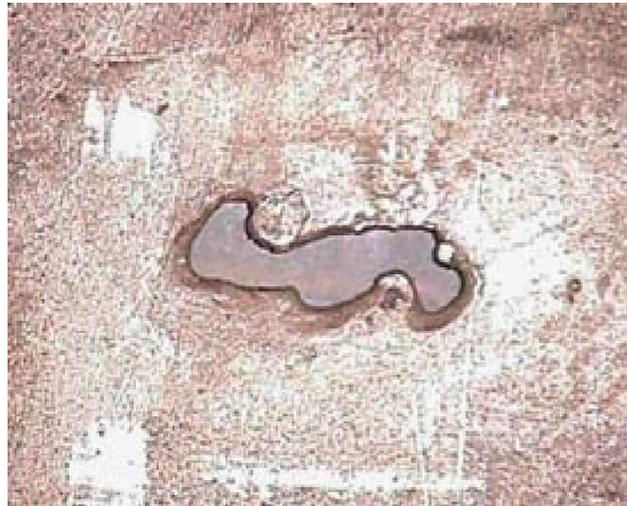
Fig.1 A sample of hole defect
