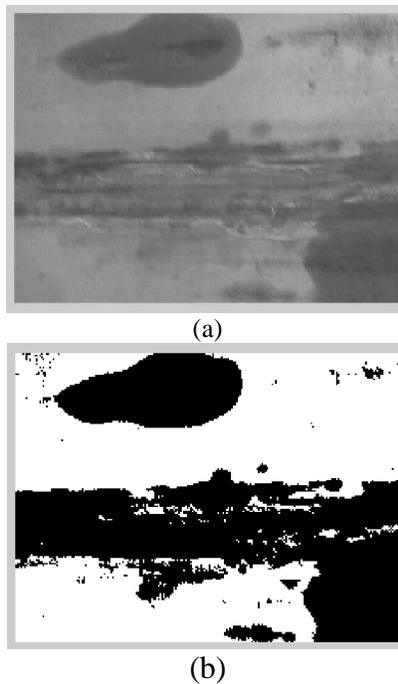
Fig.6 (a)original image of a rust defect (b)Global thresholded image of the rust defect
