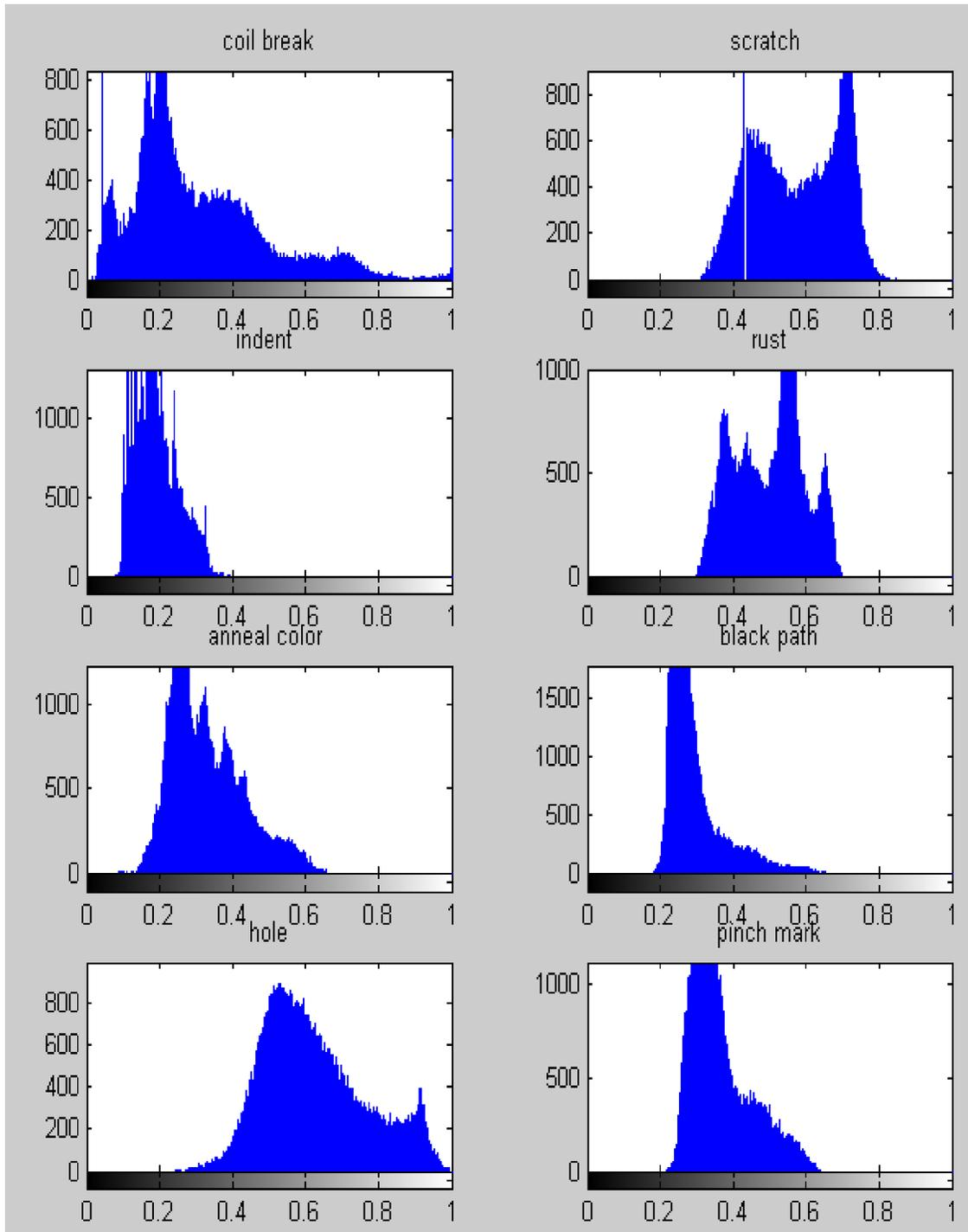
Fig.5 Comparisons of the coil break defect image histogram with the other defects
