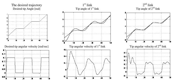
Figure (8) The simulation results of the desired trajectory of two flexible link 4.3 Fuzzy Control of Non-linear Model of Two Links Flexible Robot
