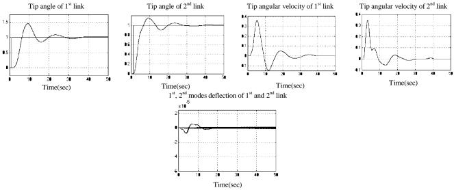
*Figure (10)* The simulation results of the fuzzy controller of non linear model of two flexible links.
