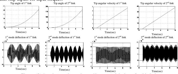
Figure (2) Simulation of open loop of linear model of two flexible links.
