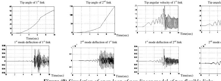
Figure (9) Simulation of open loop of non linear model of two flexible links.
